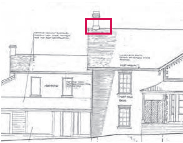
Location for inspection of flashing at western chimney. (Goering, 1982. Annotated by ERA, 2017).
